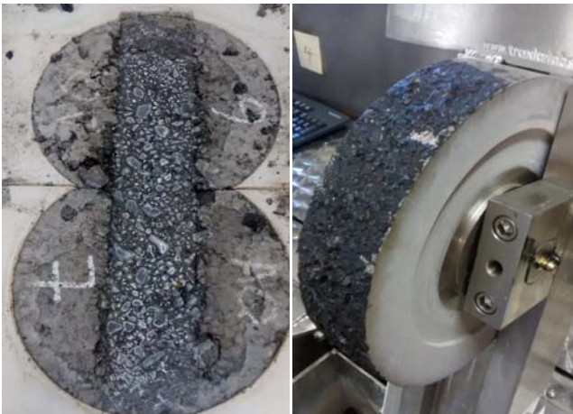
Figure 2: Photos of Aquapatch Specimens after Testing and Tire Pickup - Hamburg Test
